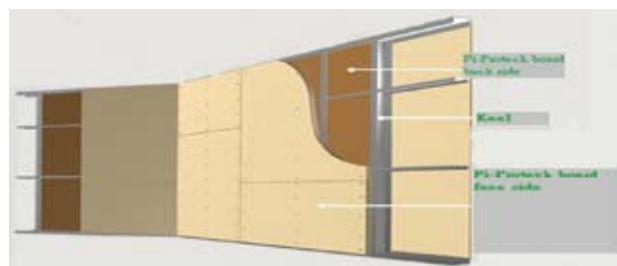
Fire-rated and insulation partition/ceiling 隔熱防火間牆及天花
