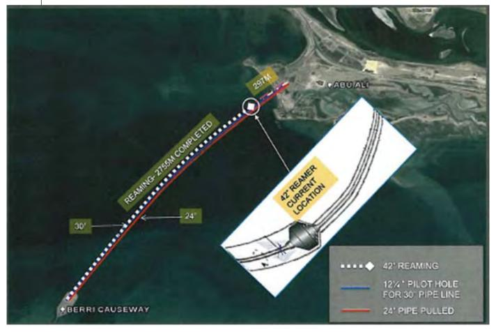
In November 2008 TT-UK were contacted by the Middle East specialist HDD Contractor Digital Connection Co Ltd of Al-Khobar, Kingdom of Saudi Arabia (KSA). They sought technical advice and assistance in the recovery of a 42" hole-opener that had become stuck along with the 3 km drill string beneath the seabed during a pre-ream pass on the sec ond of two under sea pipeline crossings.
